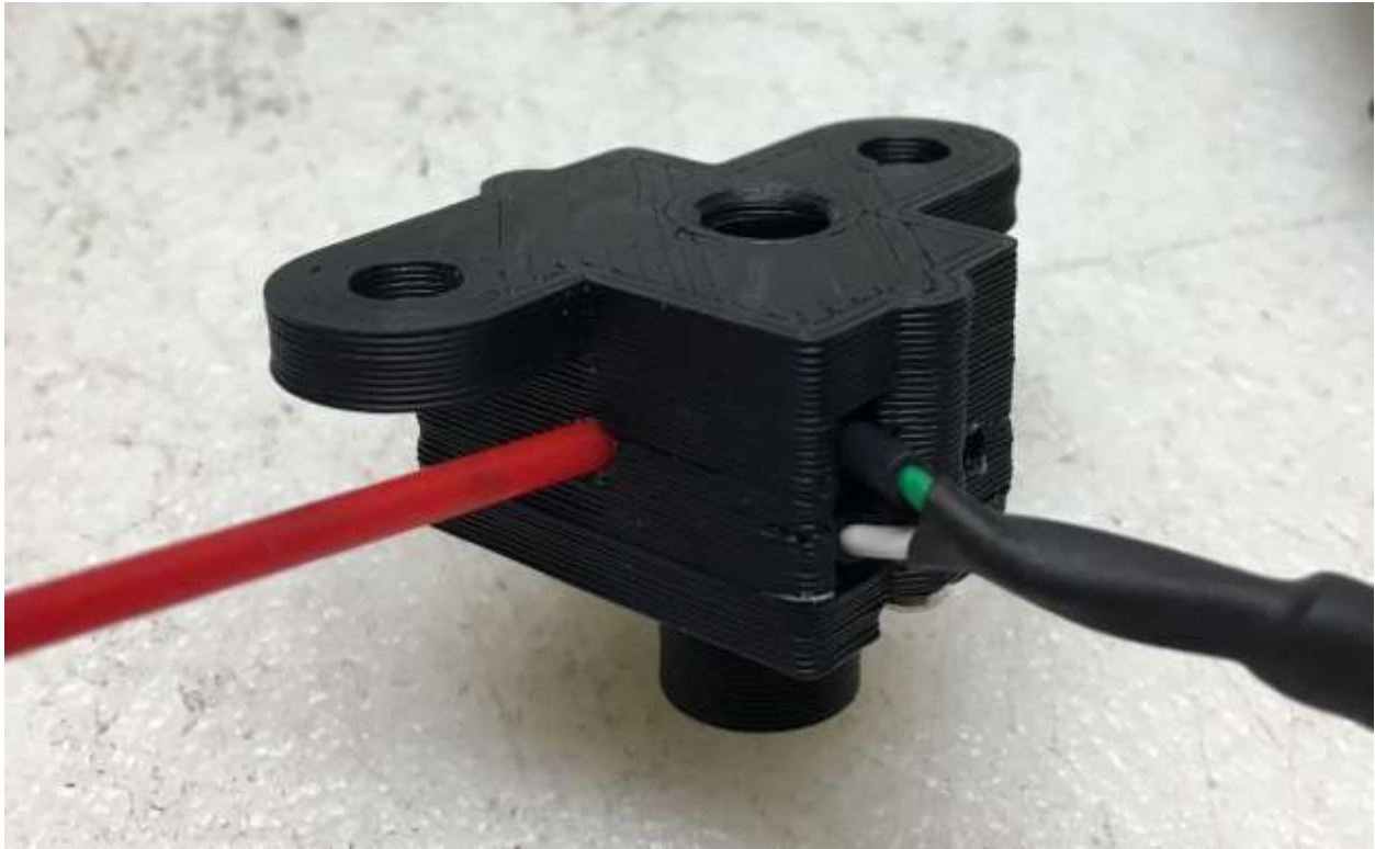
Figure 32: Blowing out decap sensor with compressed Air.
