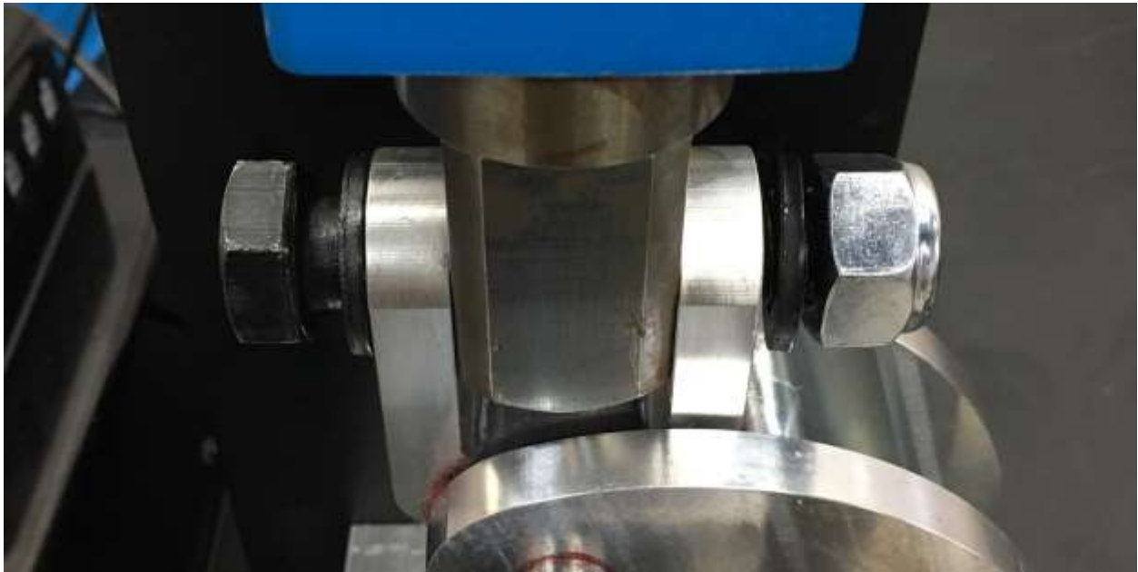
Figure 15: Inserting M14 Bolt through 650 ram (shown partially tightened)
