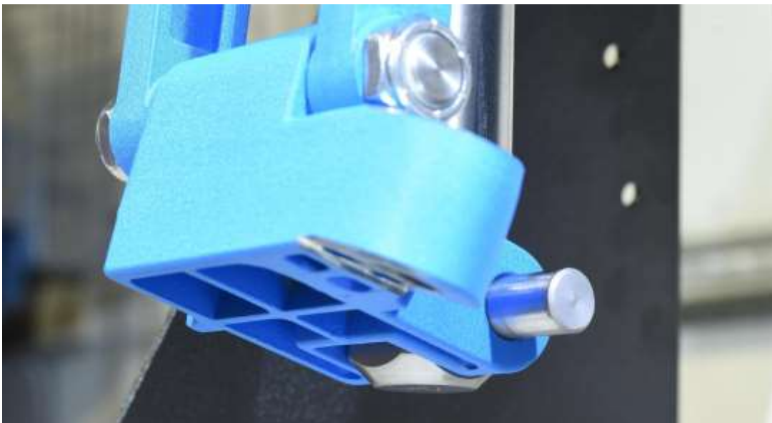
Figure 6: Removing knuckle Pin (Do not Discard Pin)
