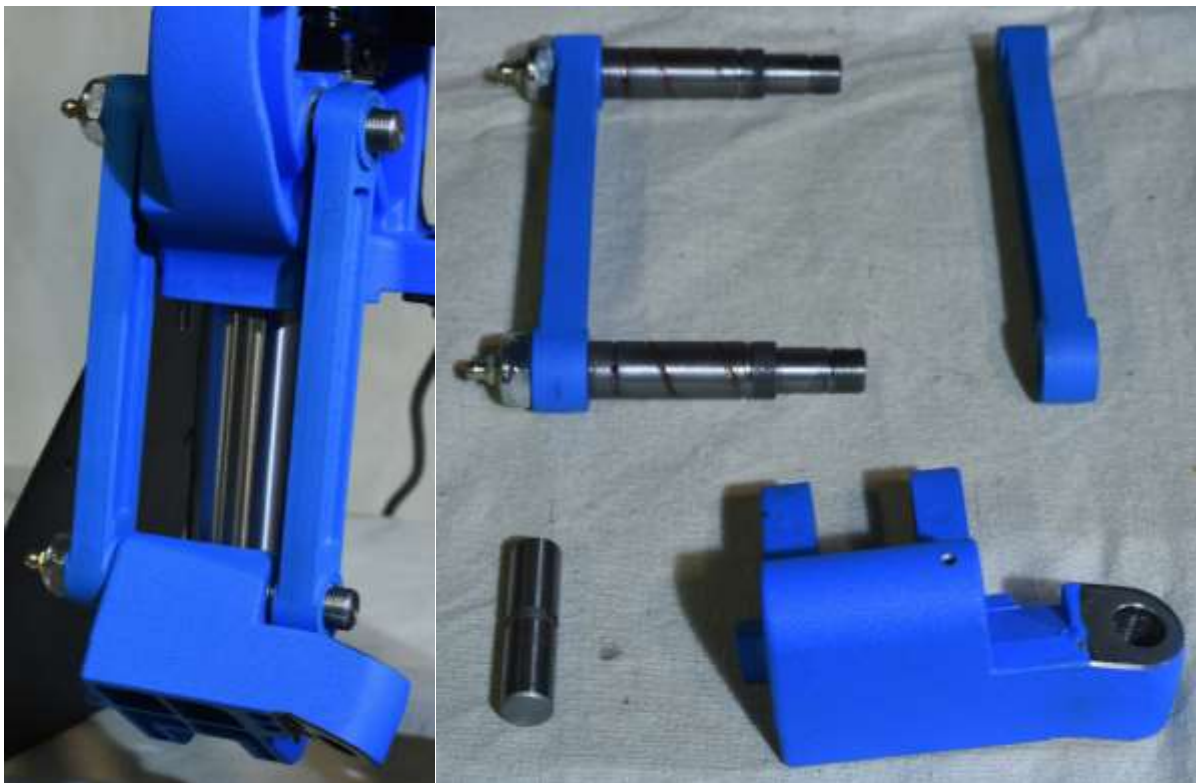
Figure 8: Link arms, knuckle and pin removed from 650.
