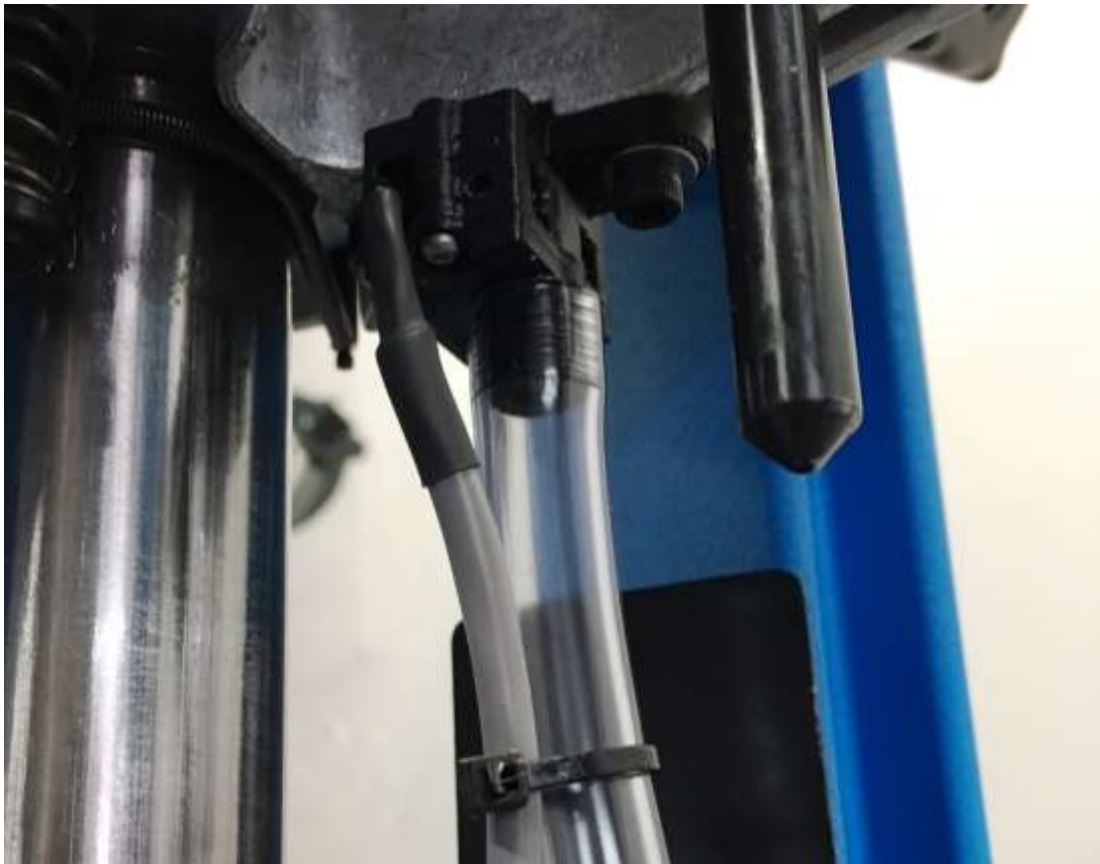
Figure 31: Decap Sensor Installed
