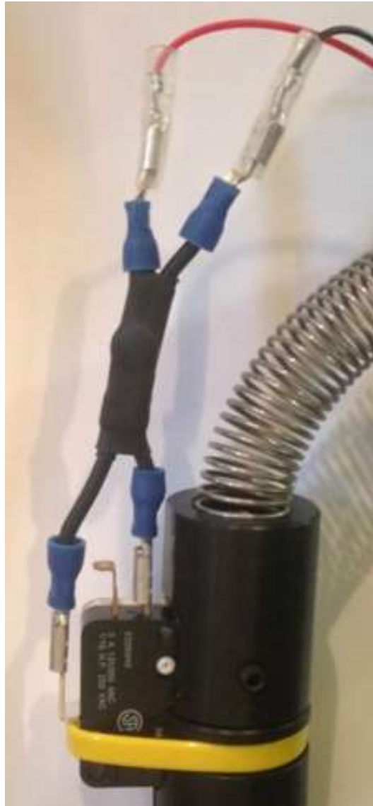
Figure 27: Filter installed on Mr. Bulletfeeder (Double Alpha)
