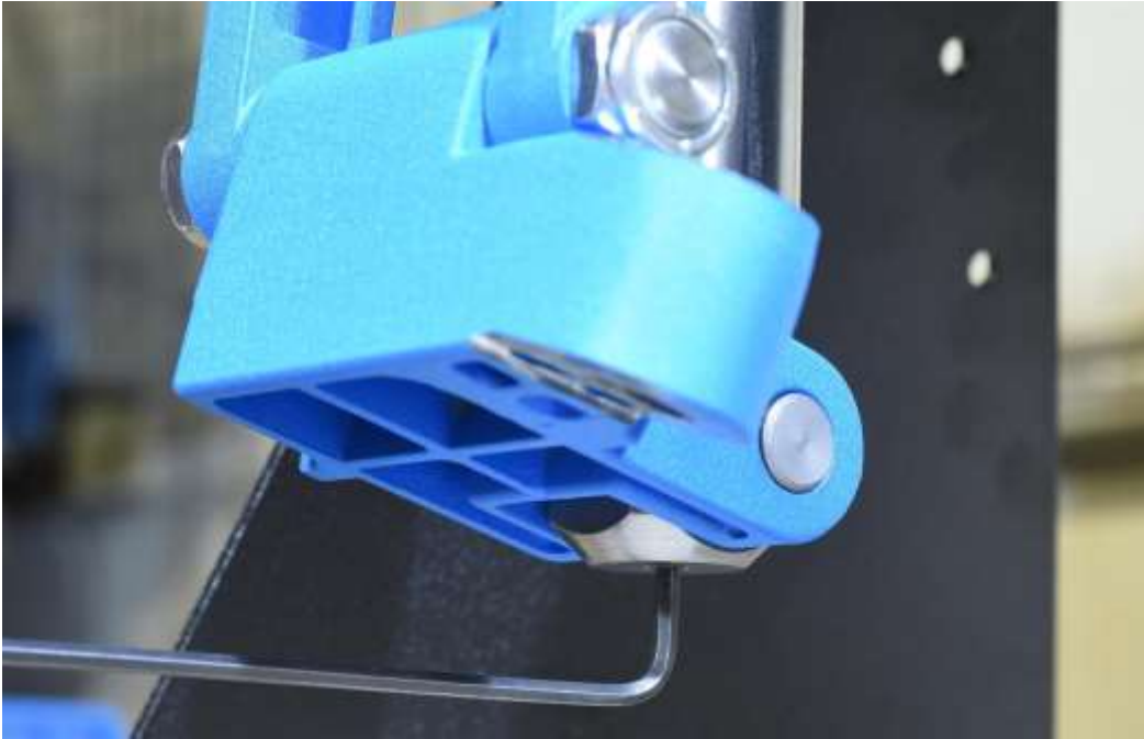
Figure 5: Removing Set screw from 650 Ram (Do not discard setscrew)
