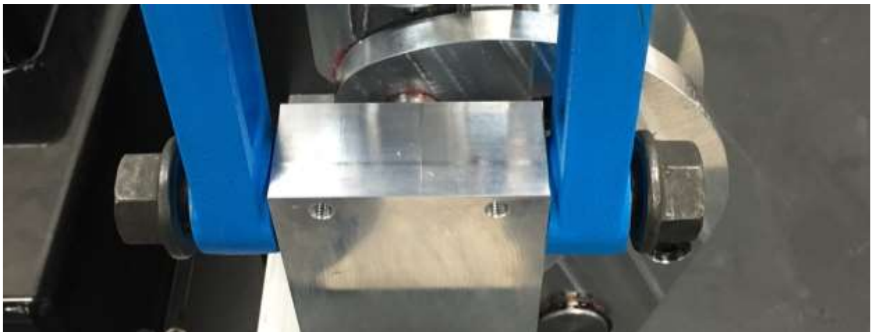
Figure 16: 1/2" hex head screws partially tightened.
