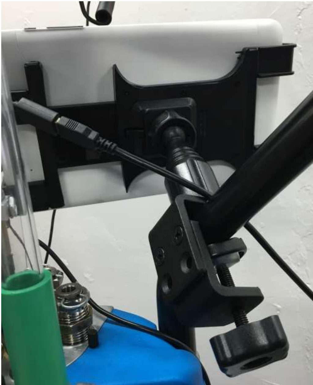
Figure 19: Recommended Tablet Mounting location (Standard 9 inch tablet shown above)
