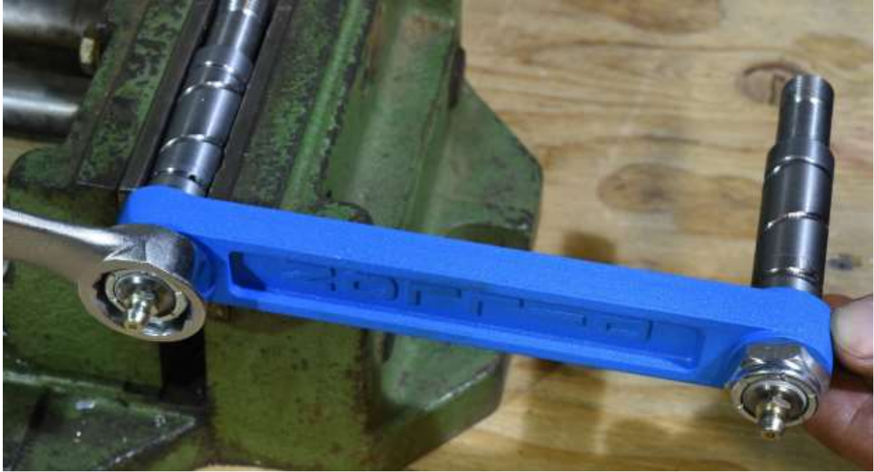
Figure 9: Removing lower pin on left side link arm
